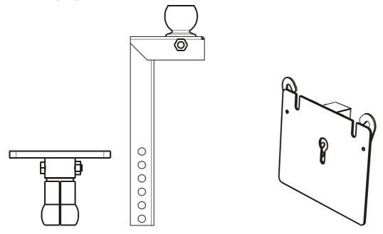
The screws to assemble the short ceiling bar are included. You will need a wrench 17mm. The screws to fix the base plate to the ceiling have to be provided on site, cf. Required tools.
